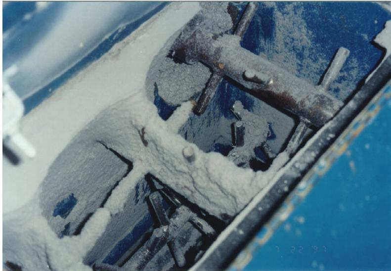
**Figure 6: Fiber Pugmill-Type Dispersion System**
