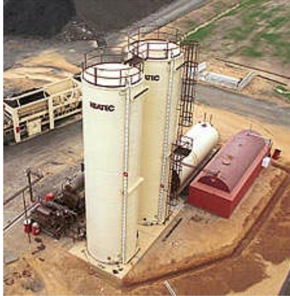
**Figure 5: Vertical Asphalt Binder Storage Tanks (Courtesy Heatec, Inc.)**
