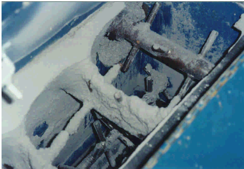
Figure 13: Fiber Pugmill-Type Dispersion System
