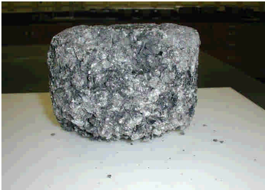
Figure A-2: Illustration of Sample after Cantabro Abrasion Test
