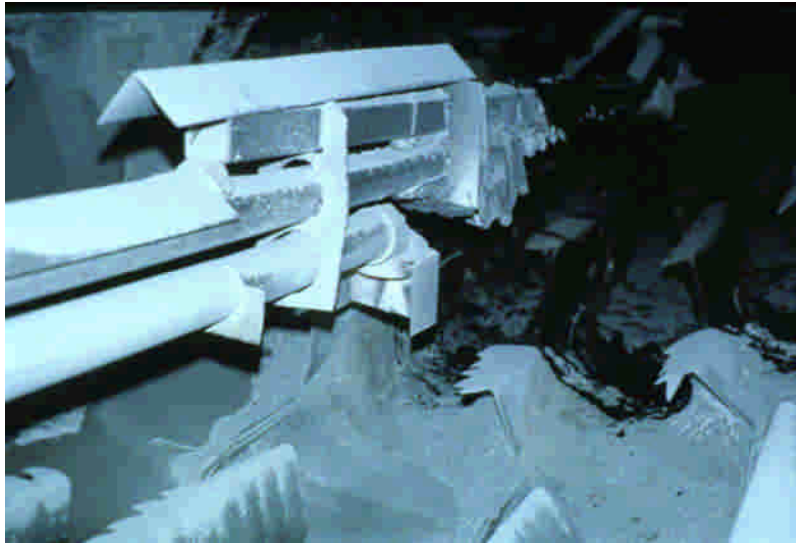
Figure 14: Fiber Injection Point in a Drier-Drum Plant
