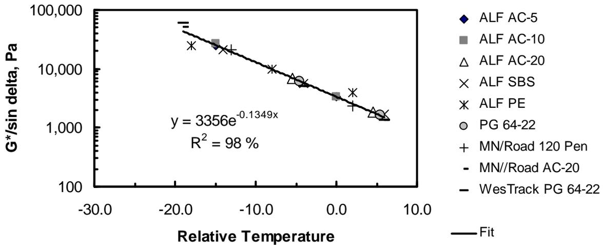
**Figure 9. Temperature Dependence of Nine Asphalt Binders Relative to the PG Grading Temperature.**
