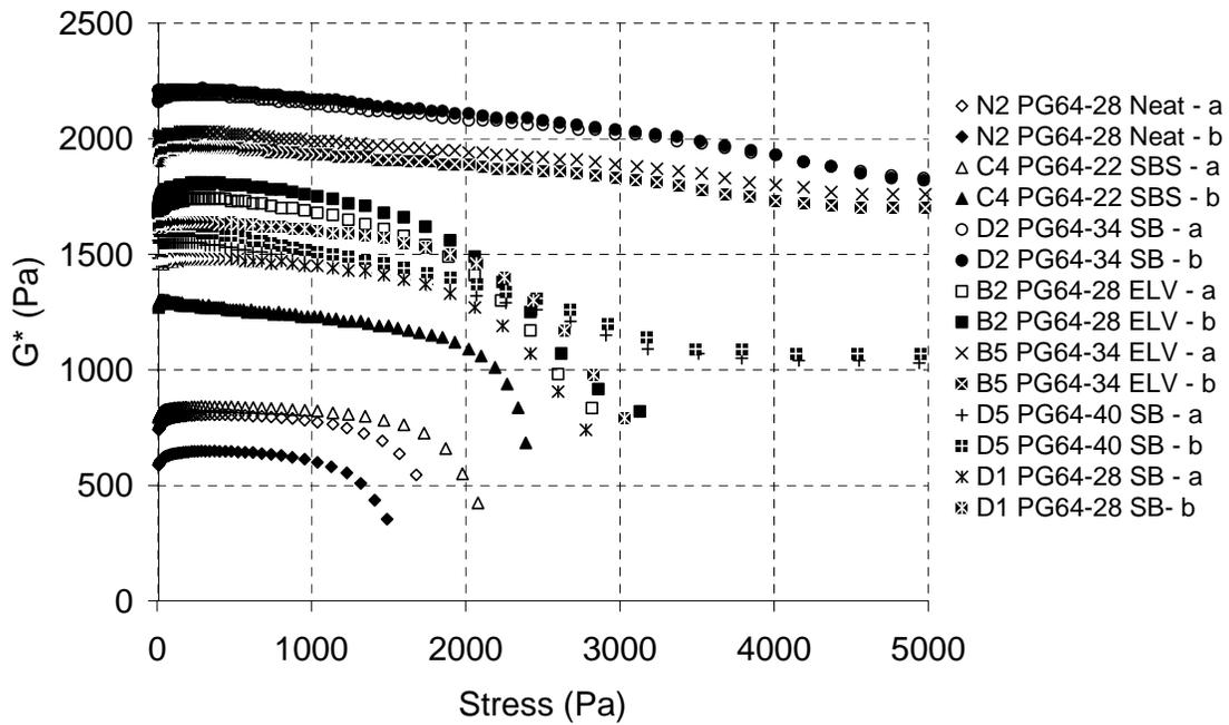
Figure 22.  $|G^*|$  at 1 Hz v/s Stress, PG64-XX Binders.
