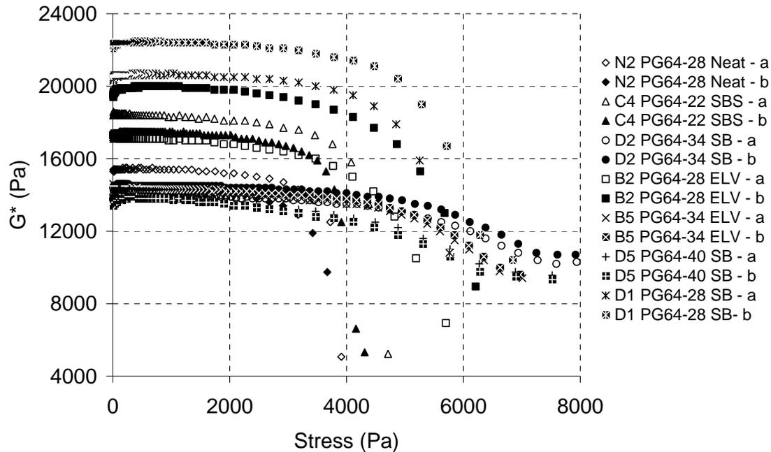
**Figure 23.  $|G^*|$  at 25 Hz v/s Stress, PG64-XX Binders.**
