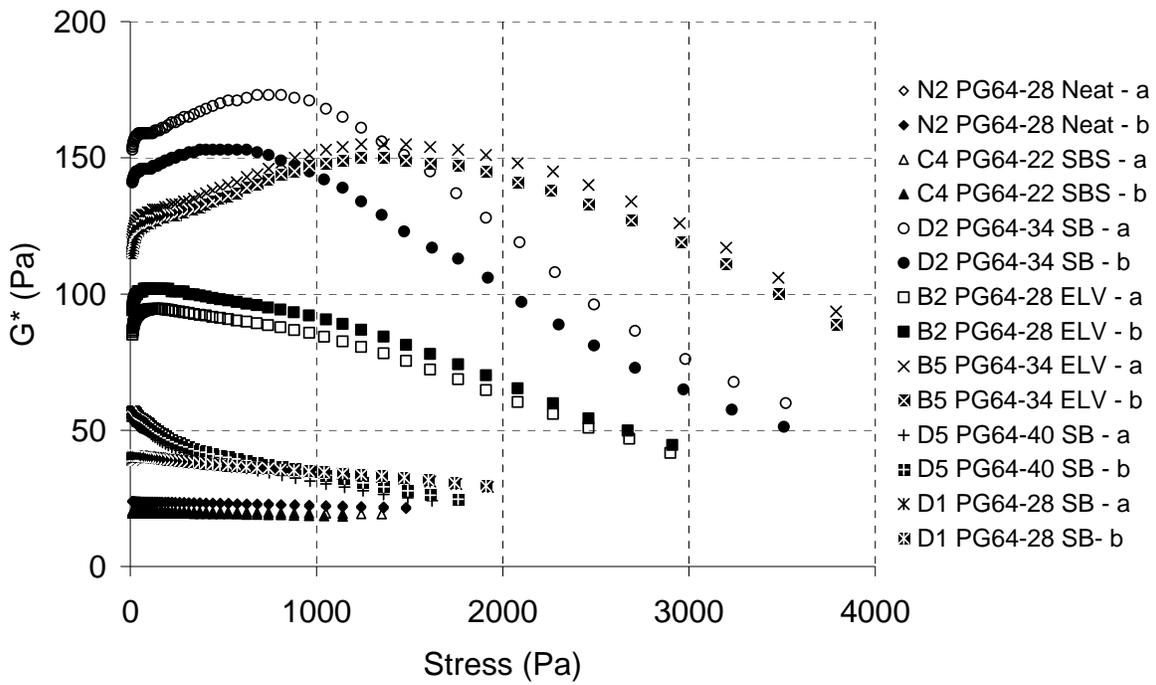
Figure 21.  $|G^*|$  at 0.01 Hz v/s Stress, PG64-XX Binders.
