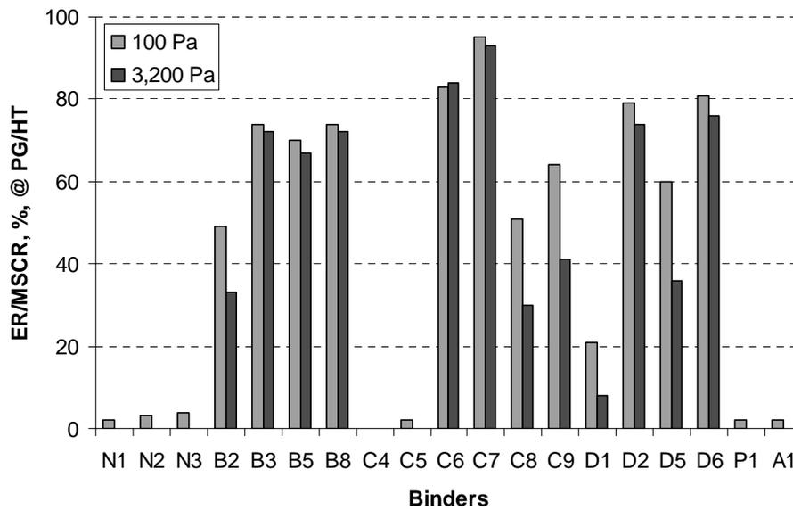
Figure 18. Comparison of ER/MSCR at PG/HT at 100 Pa and 3,200 Pa.
