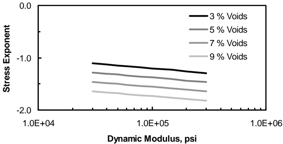
**Figure 4. Effect of Dynamic Modulus and Air Void Content on Stress Sensitivity of HMA Mixtures in the Database as Indicated by the Stress Exponent in Equation 12.**
