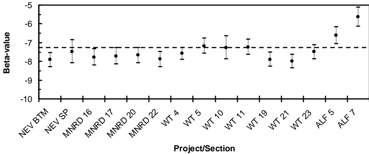
**Figure 2. Differences in Regression Constant for Project/Sections 2 through 15. Project 1 is the reference value; bands represent 2s confidence limits.**
