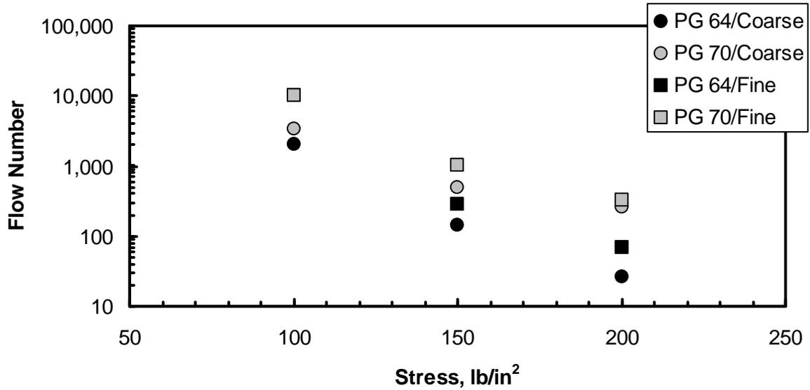
**Figure 28. Flow Number as a Function of Stress Level for Four Different Mixtures.**
