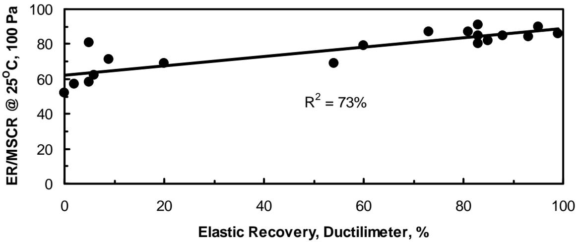
Figure 13. Elastic Recovery/MSCR at 25°C and 100 Pa as a Function of Elastic Recovery/Ductilimeter, also at 25°C.
