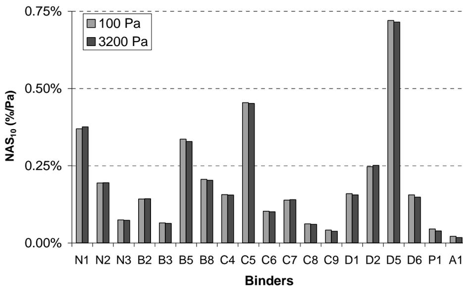
**Figure 19. Comparison of  $NAS_{10}$  at 25° at 100 Pa and 3,200 Pa**
