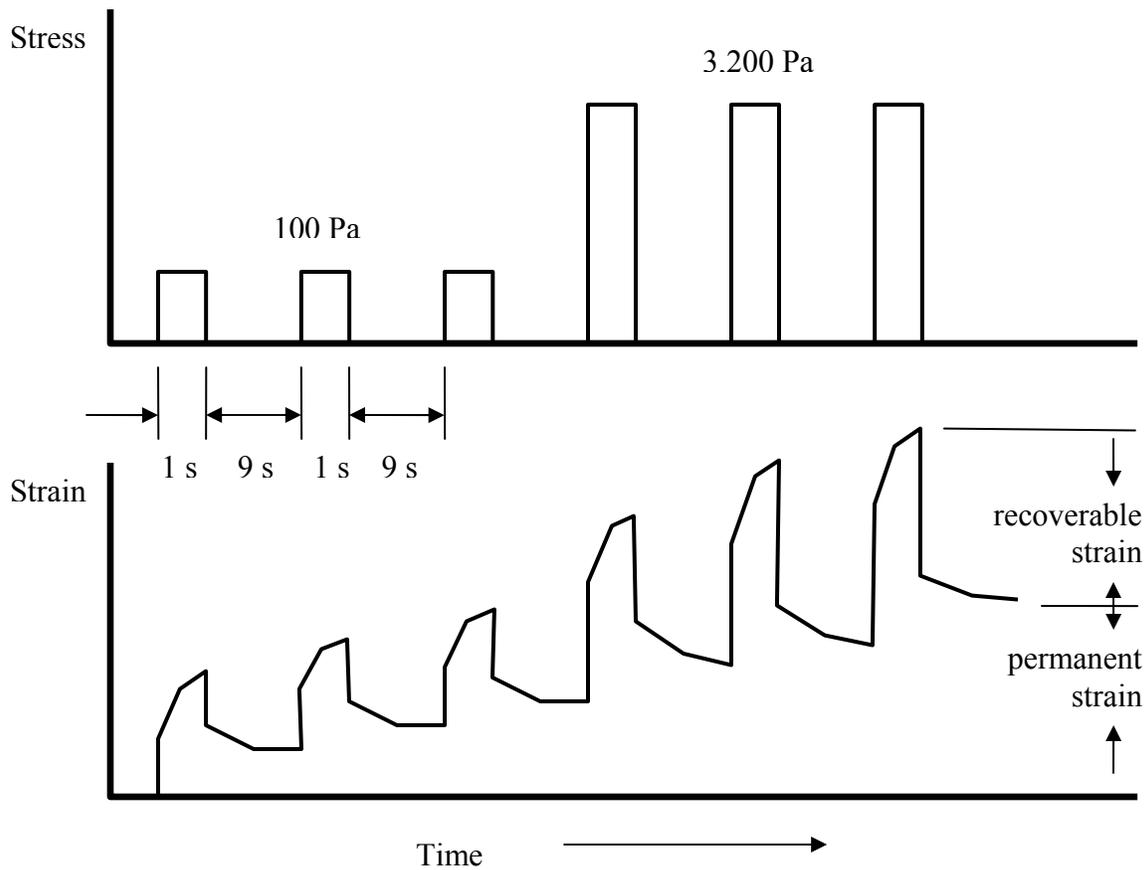
**Figure 11. Diagram of Multiple Stress Creep and Recovery Test as Proposed by the FHWA.**
