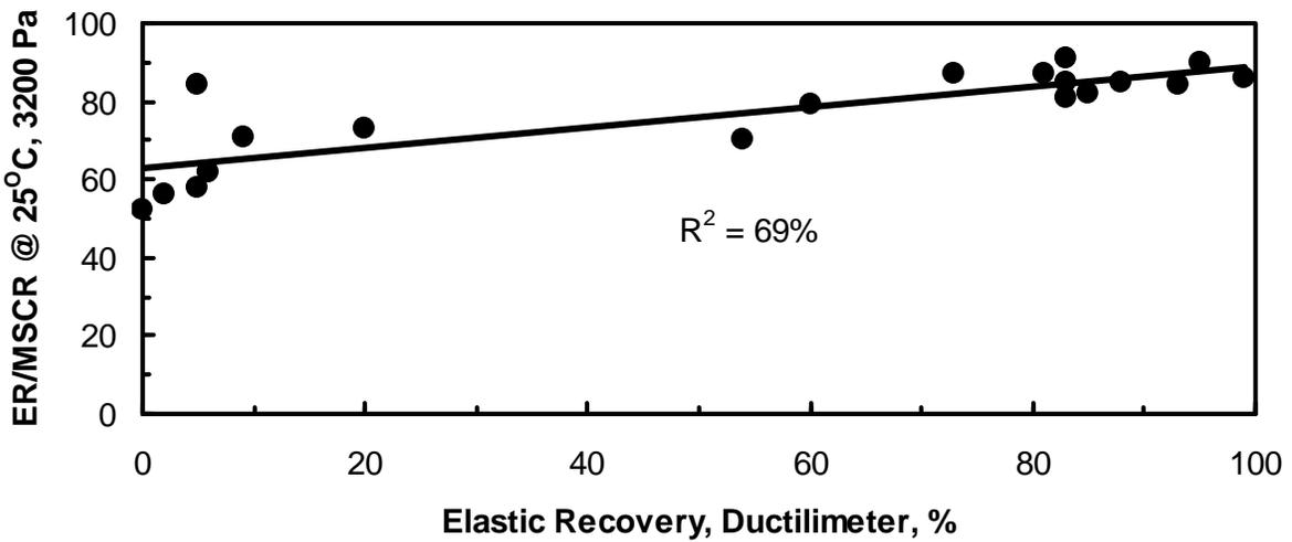
Figure 14. Elastic Recovery/MSCR at 25°C and 3,200 Pa as a Function of Elastic Recovery/Ductilimeter, also at 25°C.
