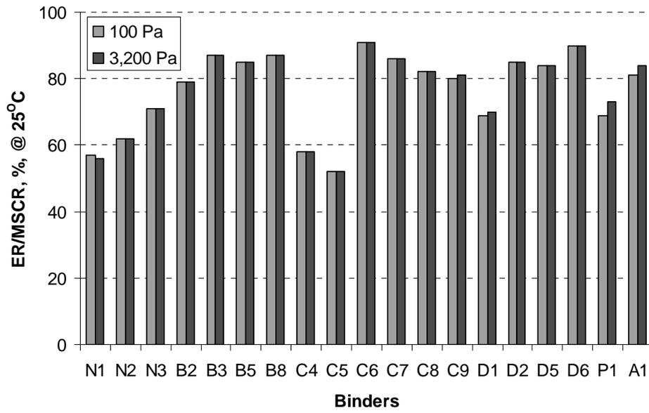
Figure 17. Comparison of ER/MSCR at 25° at 100 Pa and 3,200 Pa.
