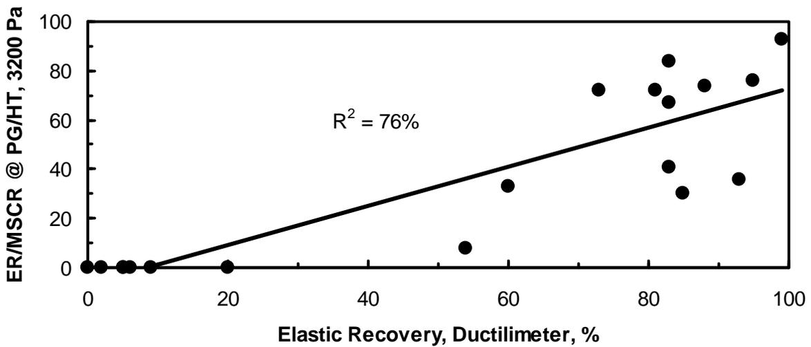
**Figure 16. Elastic Recovery/MSCR at High Grading Temperature and 3,200 Pa as a Function of Elastic Recovery/Ductilimeter at 25°C.**
