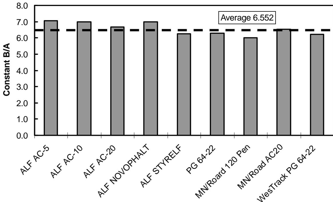
**Figure 10. Values of the Constant B/A in Equations 29 and 30 for Nine Asphalt Binders.**
