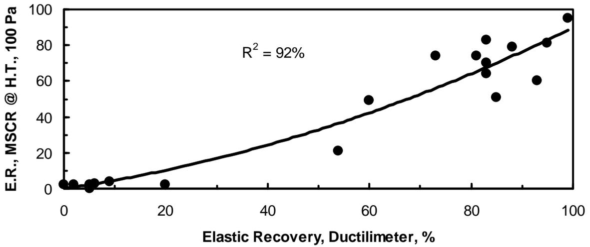
**Figure 15. Elastic Recovery/MSCR at High Grading Temperature and 100 Pa as a Function of Elastic Recovery/Ductilimeter at 25°C.**
